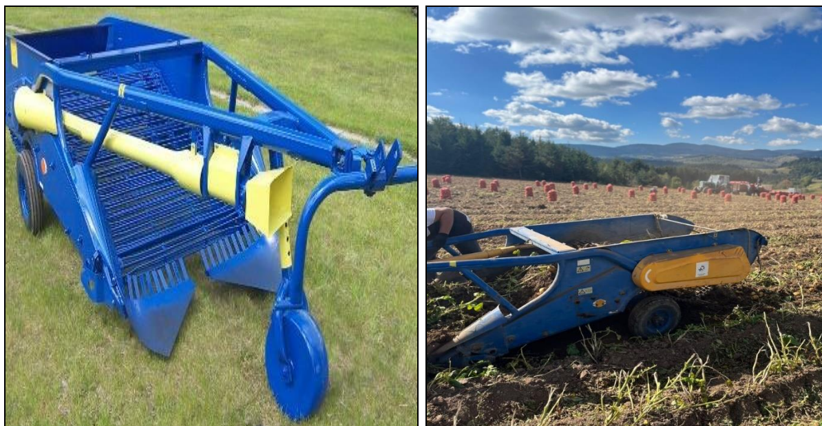
Figure 2. Rolmet two-row potato harvester (U609/0-2)
