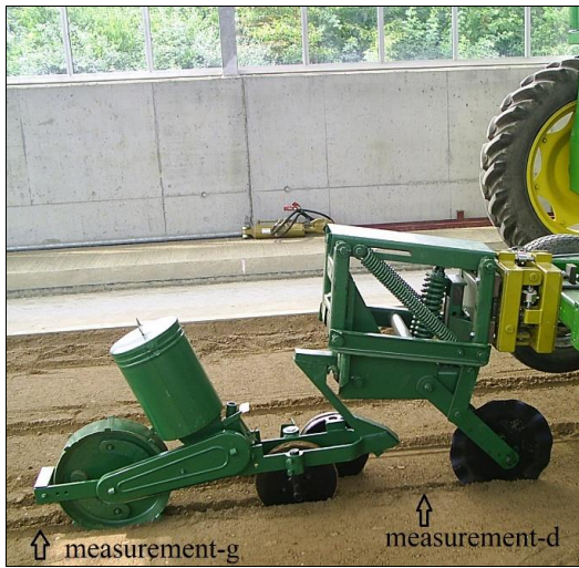
Figure 7. Experimental prototype with rifle disk
