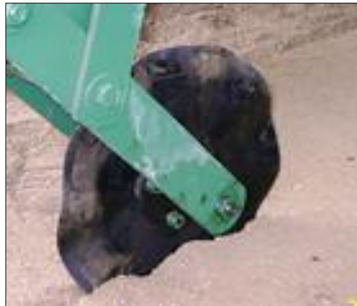
Figure 5. Corrugated disk - disk B
